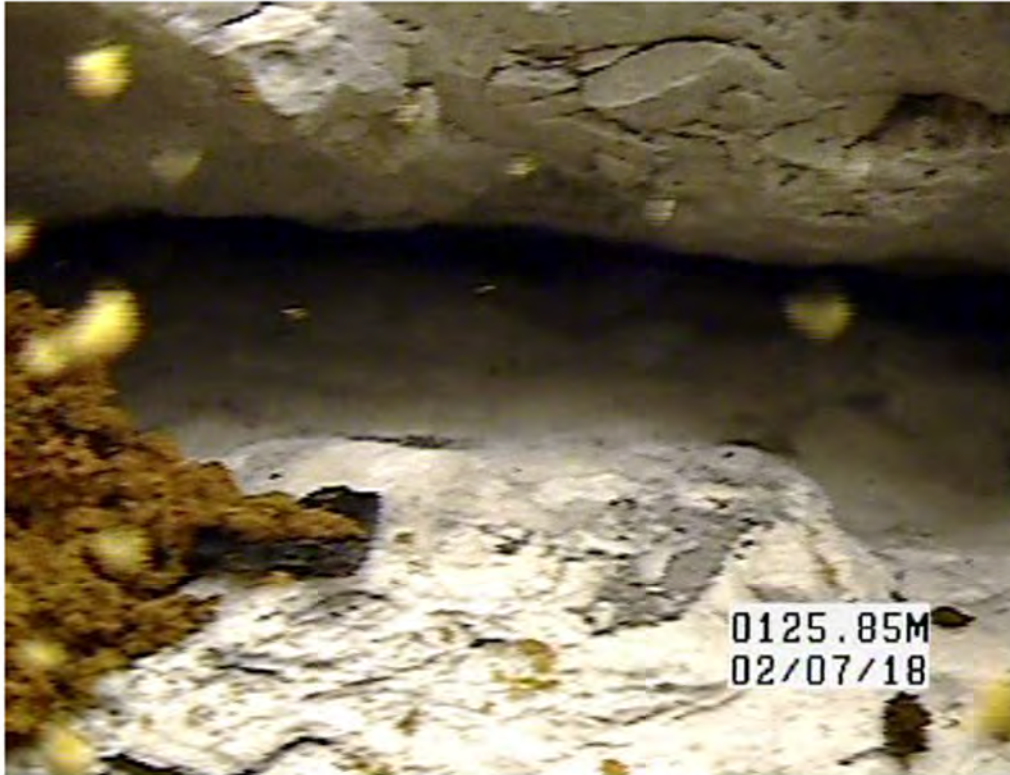
Photo 5: Likely main water producing feature near base of well with visual flow.
